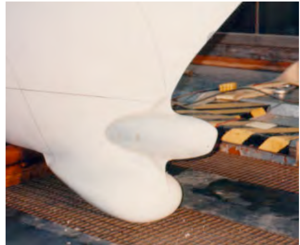
Fig. 4. Retrofit bow bulb on DDG 51 model
