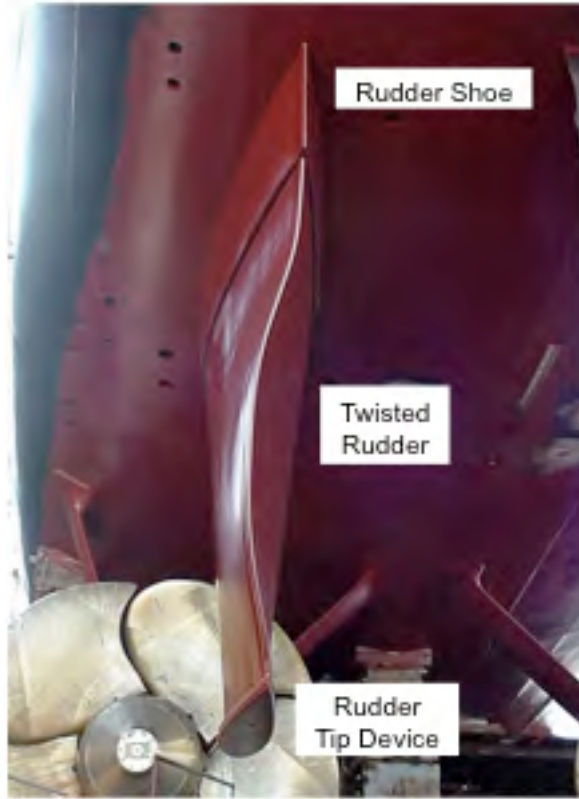
Fig. 14. Twisted rudder on BULKELEY (DDG 84)
