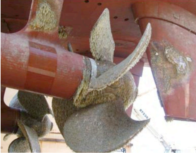
Fig. 15. Severe biofouling on STOCKDALE (DDG 106)
