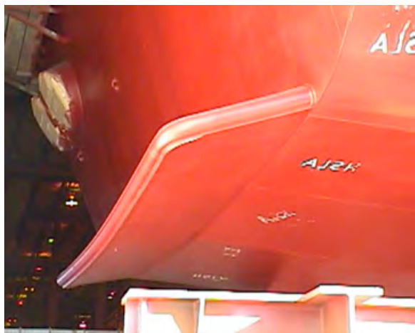
Fig. 10. DDG 79 Flight IIA stern flap on OSCAR AUSTIN (DDG 79)
