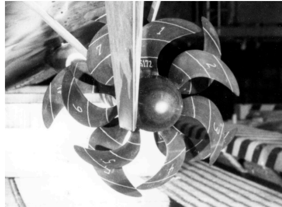
Fig. 2. DDG 51 CR-1 design model propellers
