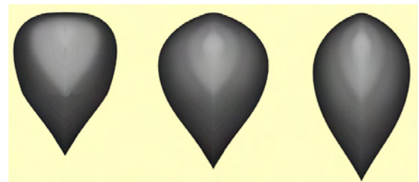
Fig. 5. Cross-section shapes of candidate bow bulbs
