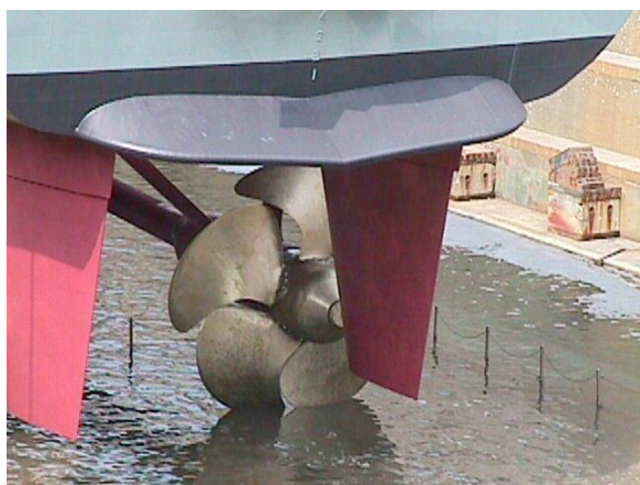
Fig. 11. DDG 51 Flight I/II retrofit stern flap on CURTIS WILBUR (DDG 54)
