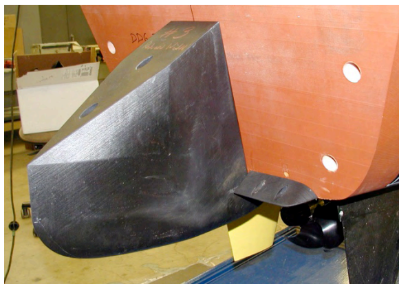
Fig. 7. DDG 51 Phase I Stern end bulb with stern flap installed on model
