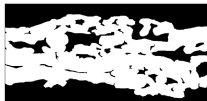
Fig. 11. Cross sectional geometry of a paper sheet. Manual pore volume detection by binarization (b) of a microscope image (a). Some fibers are cut longitudinally, and they move at some point out-of-plane. It is assumed that they are still close to the cutting plane, and therefore this region is not accounted for as pore volume.
