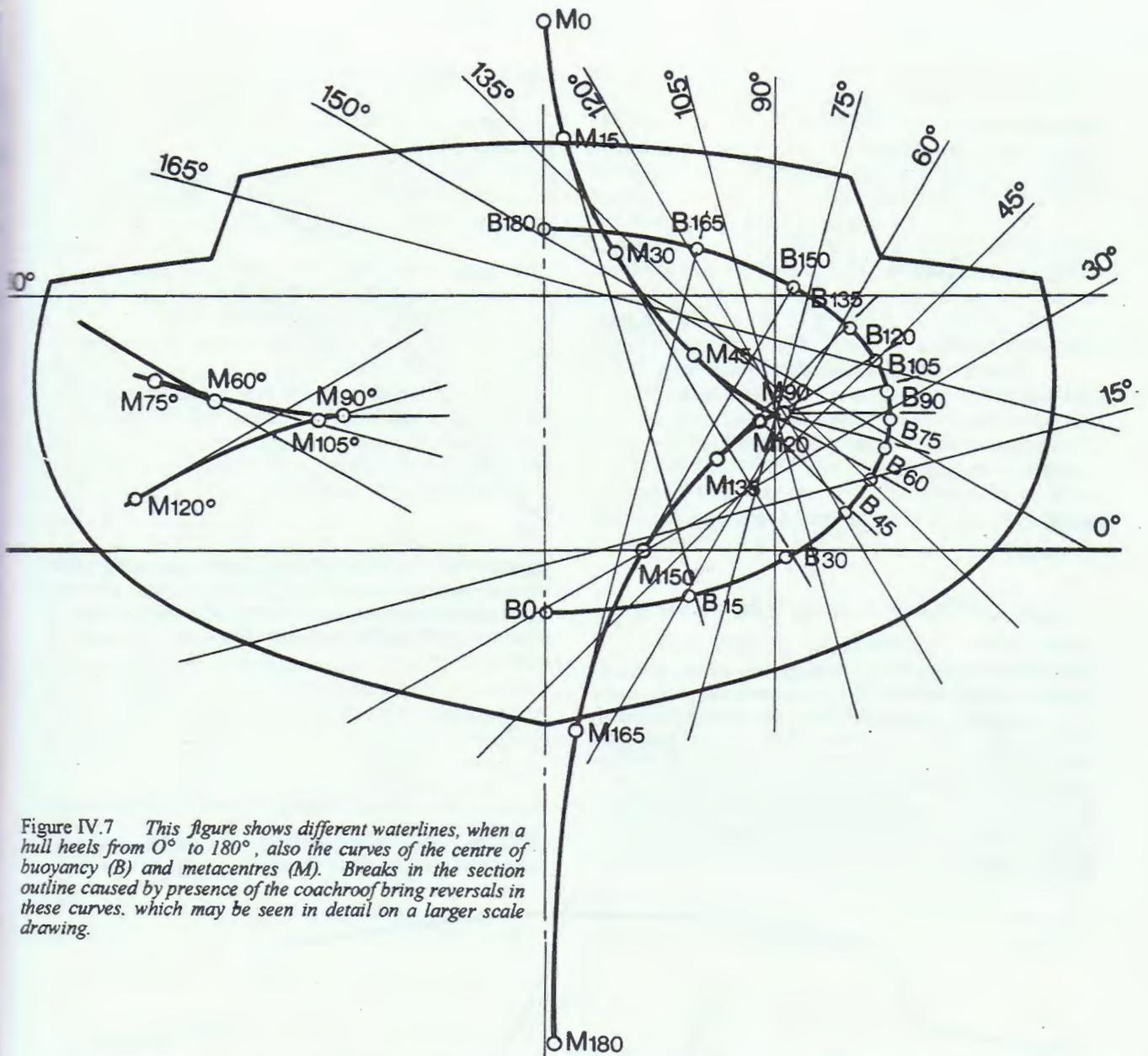
Figure IV.7 This figure shows different waterlines, when a hull heels from  $0^\circ$  to  $180^\circ$ , also the curves of the centre of buoyancy (B) and metacentres (M). Breaks in the section outline caused by presence of the coachroof bring reversals in these curves, which may be seen in detail on a larger scale drawing.
