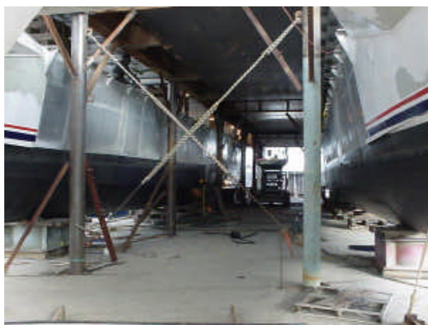
Fig. 1 M/V JET CAT EXPRESS under repair with the superstructure raised.
