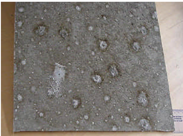
Fig. 4 M/V JET CAT EXPRESS - Pitting in a section of spray rail. This plate was in service for less than eight months
