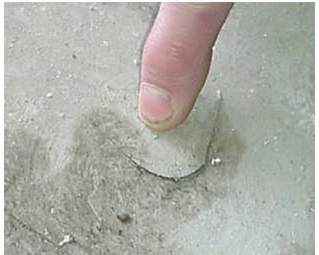
Fig. 3 M/V JET CAT EXPRESS - Deck plating showing a section about to pop out
