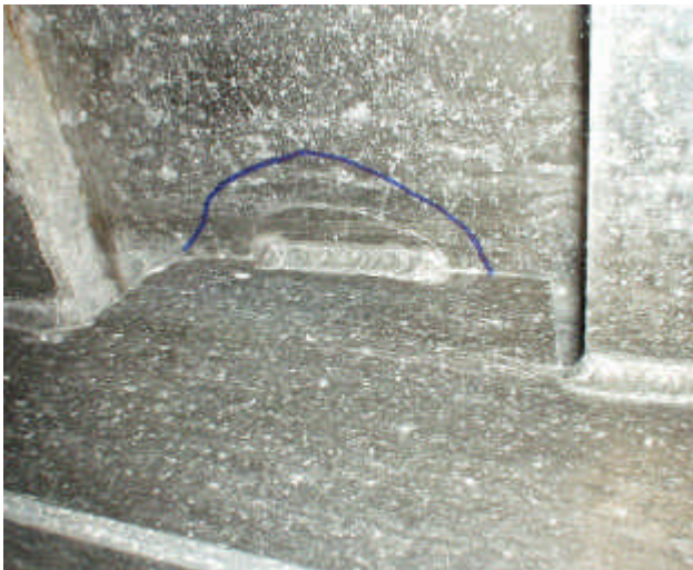
Fig. 2 M/V HULA KAI - Stress corrosion cracking often referred to as "Smiley face cracks"
