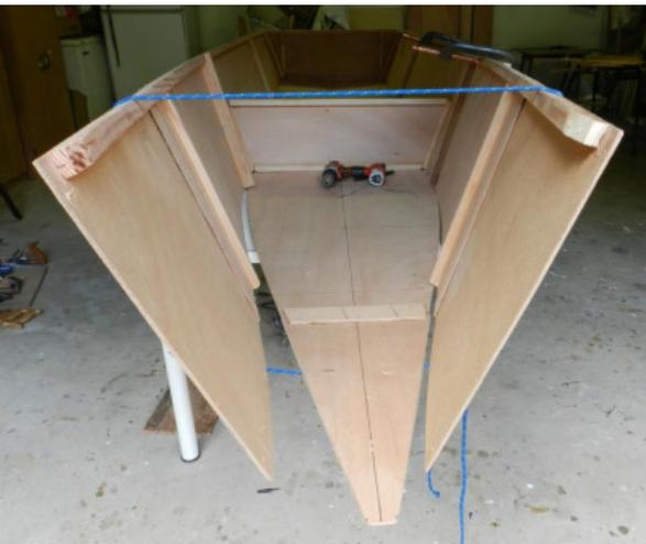
The bow is the tricky area as it is important that it is vertical and that the hull is not twisted.
