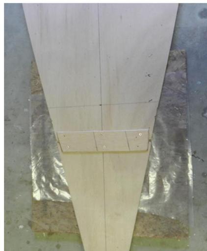
Glue butt straps in position to join the panels
