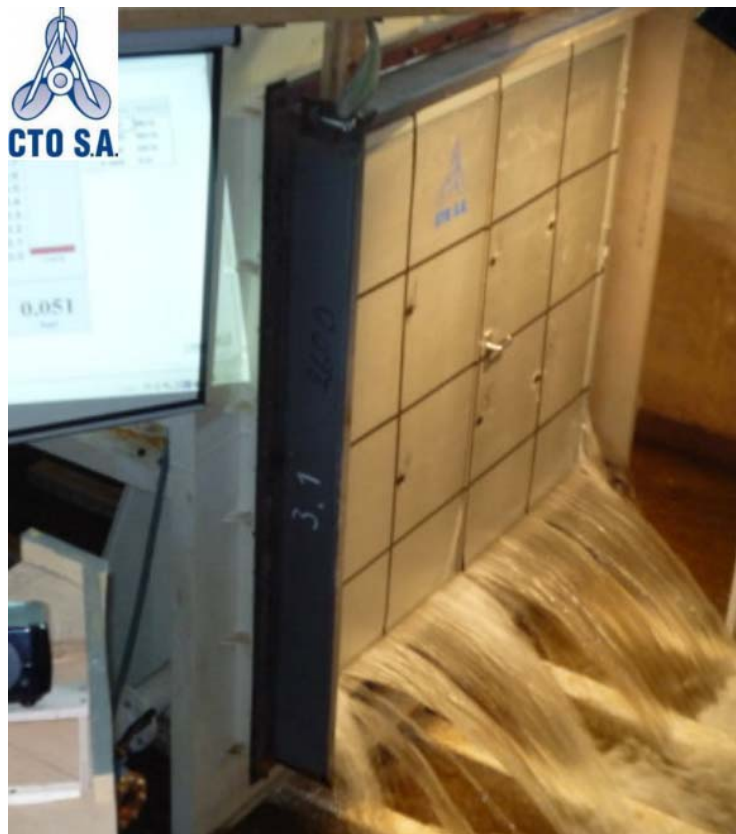
Figure 11. A-60 double leaf hinged marine fire door leaking (FLOODSTAND – Integrated Flooding Control and Standard for Stability and Crises Management / CTO S.A.)
