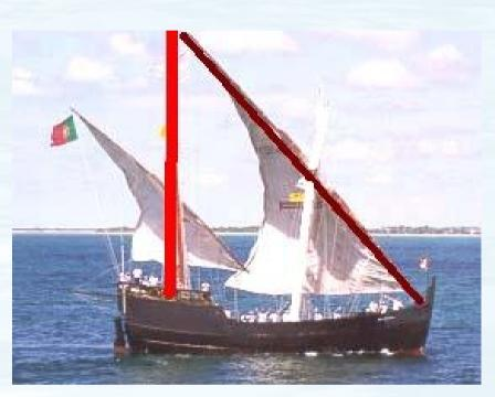
With the mast in the back, there is no mast in the way. The sail is self-tacking. A spar in the foot holds a better shape than a lateen.
