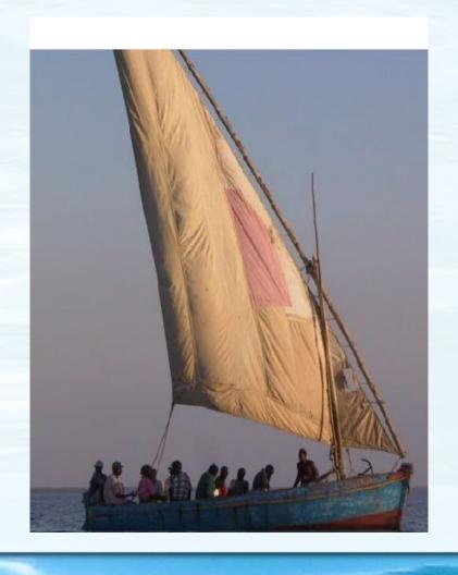
The wind on this tack is pressing the sail up against the mast. That is not good, hence the term the bad tack.
