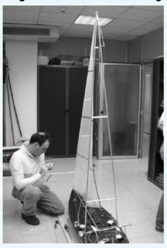
Italian researches compared a scale model A-frame aft-mast rig against a scale model race winning Bermuda rig.
