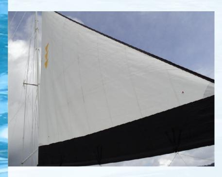
The sail of my boat is shown with the 1<sup>st</sup> trial mast. The 14mm Dyneema bolt rope both supports sail and serves like a spar. A spar within the foot helps with shape and helps channel air upwards. The 2<sup>nd</sup> mast is 18 feet shorter.
