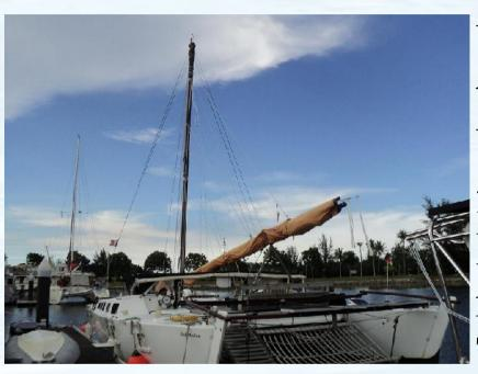
Wakataitea's owners love their rig! This James Wharram designed rig features a crab claw sail. It is located behind the mast and has two spars. The rig uses a relatively short wooden mast held up by synthetic rope.
