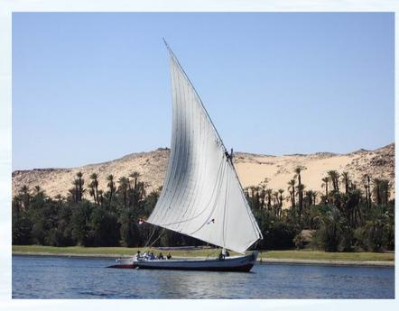
If the boat doesn't have to tack, a spar in the foot is possible and can raised on the mast's good tack.
