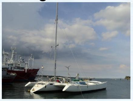
24% shorter, HOT BuOYS new rotating wing mast supports one efficient lifting sail. It has a dynamic compounded backstay.
