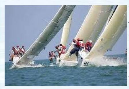
The wind's force on the Bermuda rig for the left sailboat has driven the bow almost below the waterline. Most of the wind is being spilled. Would a lifting rig be safer?.
