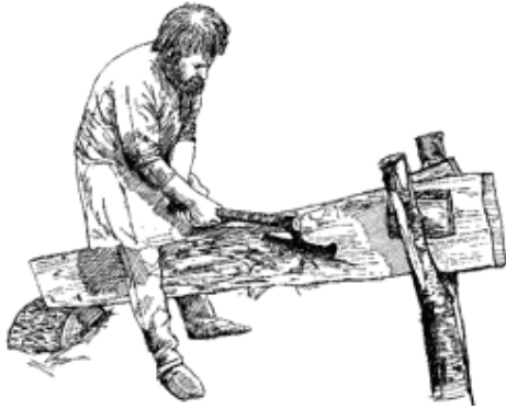
A Sideaxe in use. The strake is wedged upright so that the axe can be used in the vertical plane.
