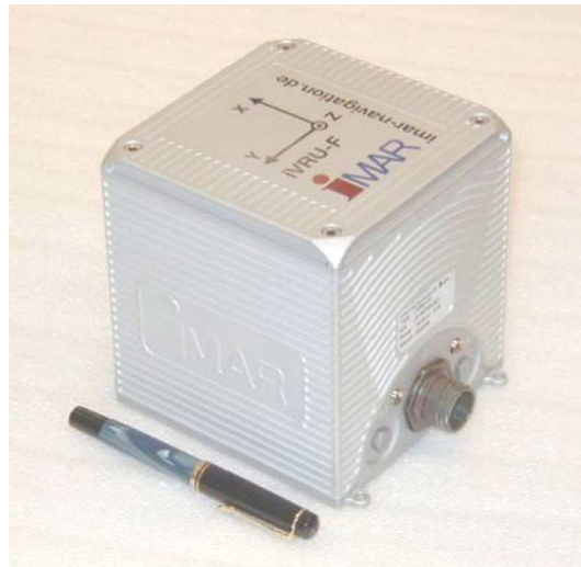
Figure 8: Inertial Measurement Unit used in Laboratory on Naval Architecture at TUHH
