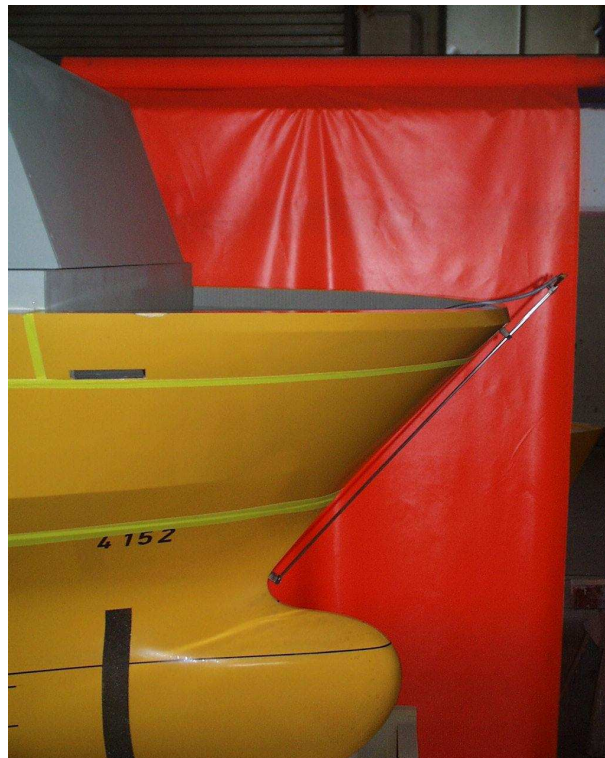
Figure 5: Resistive wave probe mounted in front of a model's bow
