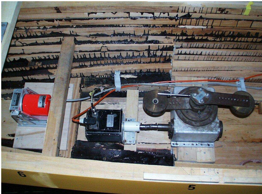
Figure 10: Counterrotating masses for roll damping test within a ship model
