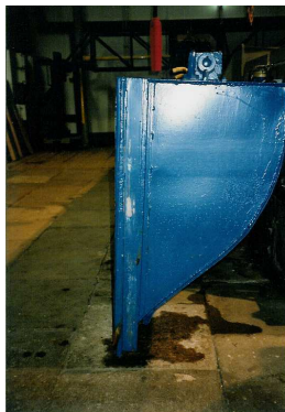
Figure 2: Plunger of the small HSVA Towing Tank
