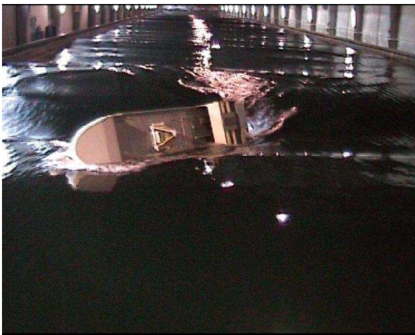
Figure 15: Capsizing of an intact RoRo vessel
