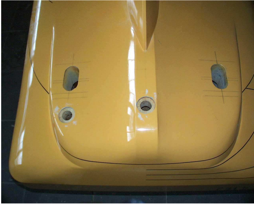
Figure 11: Holes for pressure probes (circular) and pods (oval)
