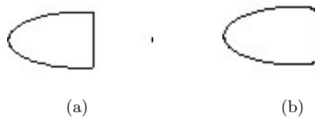
FIGURE 7. Masts for upwind tests: (a) Cut-off ellipse, (b) Cut-off ellipse, rounded edges. Source: Team New Zealand
