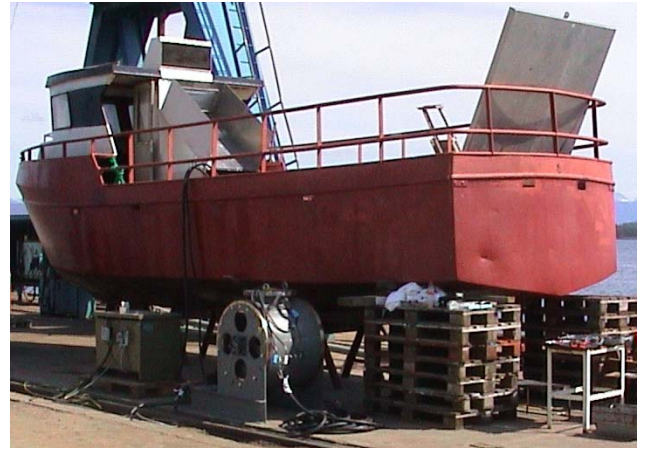
Fig 7, The boat used for testing. The thruster is in front of the picture, not yet mounted.
