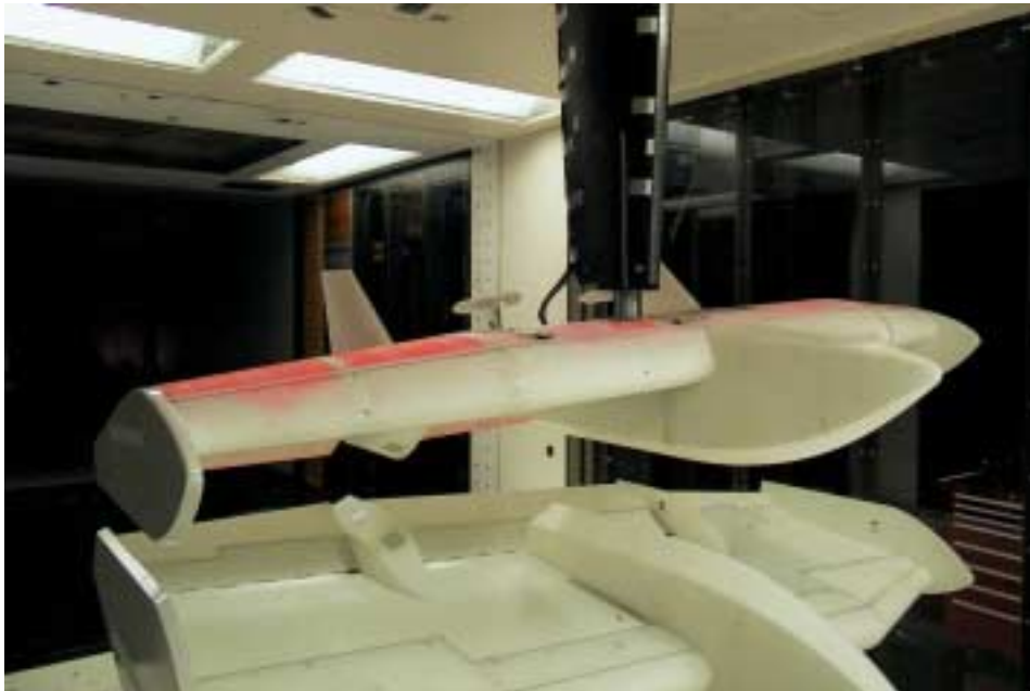
Fig. 5 Seabus wind tunnel models with 30° flap deflection
